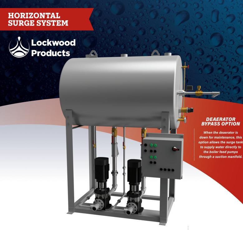
Lockwood surge systems are packaged, atmospheric-pressure, storage tanks built for commercial or industrial steam systems. The storage tank blends makeup water and condensate returns before being pumped to the deaerator. The tank is elevated over the transfer pump(s) to provide sufficient NPSH for water temperatures up to 200°F. Vertical, multistage, centrifugal transfer pumps are typically utilized since they are common in the boiler room.
